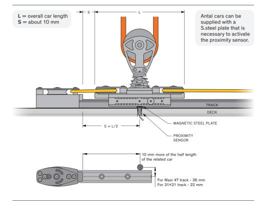
For mounting the proximity sensor drill a 16 mm hole and use silicon under the sensor cap.
