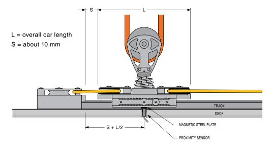
Antal cars can be supplied with a s.steel plate that is necessary to activate the proximity sensor.
