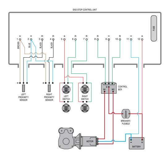
$\triangle$  If the motor turns in the wrong direction exchange 8 with 10; never exchange 3 with 4 or 6 with 7 !
